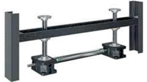
Attention must be paid to the parallelism and correct angular relationships of mounting surfaces, gears, nuts and guides to each other. The same applies for exact alignment of gears, pedestal bearings, connecting shafts and motors to each other. We recommend aligning with the help of a precision machine spirit level.
