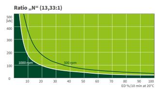
These curves are for guidance under standard industrial conditions (ambient temperature 20°C etc.) and correct maintenance (lubrication etc.). They are based on the ZIMM standard trapezoidal thread Tr 120x16. The operation cycles can be many times longer, when using ball screws.
